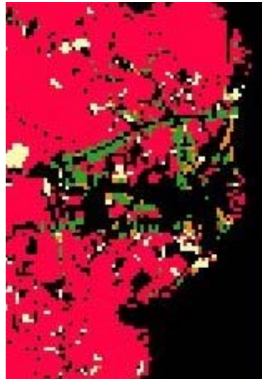
Figure 1. Comparison between real data and simulation results with a cell size of 30x30 m. Red cells: non-urban land, black cells: urban land in 1995, yellow cells: urban land in 2003 unpredicted by the model, green cells: wrong predictions, orange cells: correct predictions of the model.
